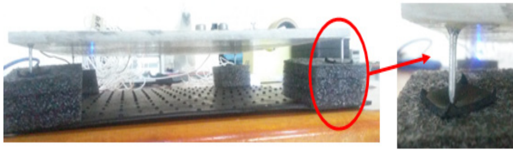
Figure 4. Glass-fibre plate pivoted by cushioned nails.
