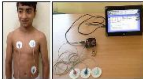
Figure 4. ECG Electrodes placements
