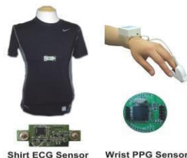
Fig. 1. Wearable health sensors with a PCB board: (a) shirt ECG sensor. (b) wrist PPG sensor
