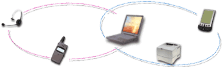
Figure 2: A Bluetooth scatternet comprises a group of piconets that have overlapping coverage
