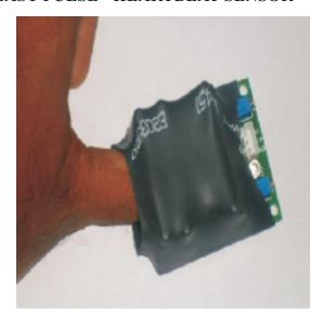
The new version uses the TCRT1000 reflective optical sensor for photo plethysmography. The use of TCRT100 simplifies the build process of the sensor part of the project as both the infrared light emitter diode and the detector are arranged side by side in a leaded package, thus blocking the surrounding ambient light, which could otherwise affect the sensor performance
