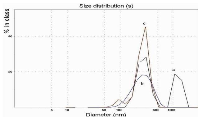
**Figure 1.** Particle size distribution plot for iron oxide pre-pared using a. alginate, b. chitosan and c. starch at disaccharide: Fe ratio of 1: 4 and at a temperature of 800°C and rate of heating of 5°C/min for a dwell time of 120 min.
