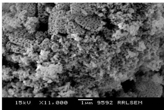
Figure 3. Scanning electron micrograph of iron oxide particles generated with chitosan template (chitosan : Fe 1 : 4).
