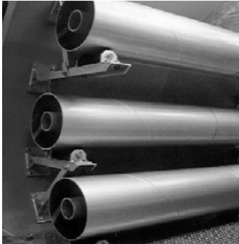
Figure 2. GIL cross section (3 phases).
