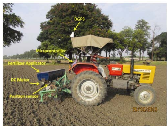
Figure 7. Field testing of digital map-based VRFA system.
