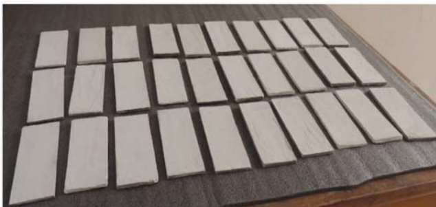
Figure 2. White cement panels for UV test.
