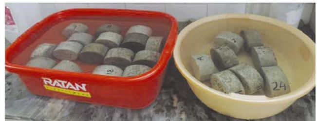
Figure 4. Concrete cores immersed in water up to 48 h (ASTM D 6489-99).
