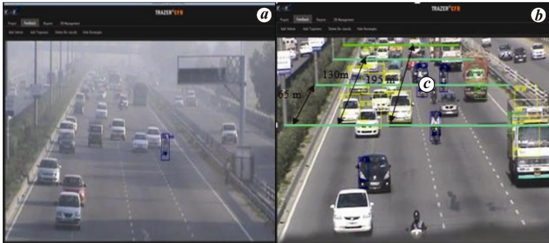
**Figure 2.** *a*, Snapshot of TRAZER detection window during fog. *b*, Different trap lengths marked on detection window.
