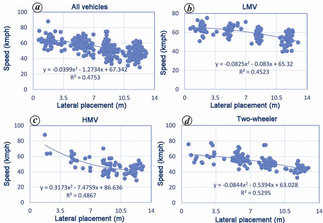
**Figure 12.** Relationship between individual vehicle speeds of (a) all vehicles with lateral placement, (b) LMV with lateral placement, (c) HMV with lateral placement and (d) two-wheelers with lateral placement.
