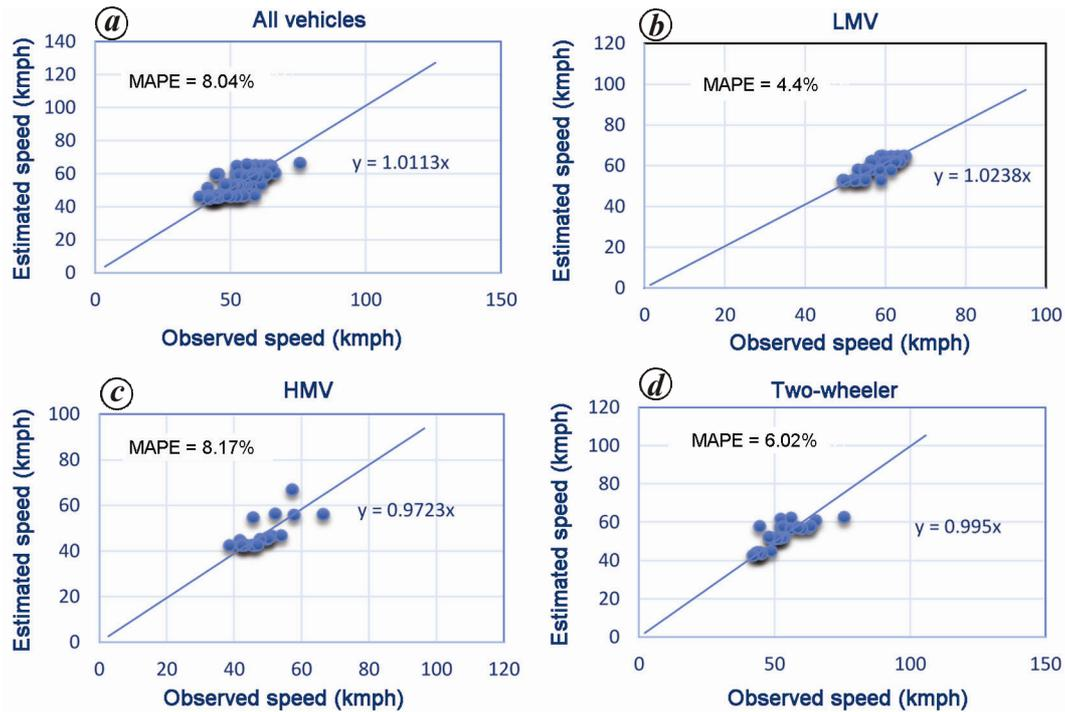
**Figure 13.** Comparison of actual and estimated values for (a) aggregate, (b) LMV, (c) HMV and (d) motorized two-wheelers.
