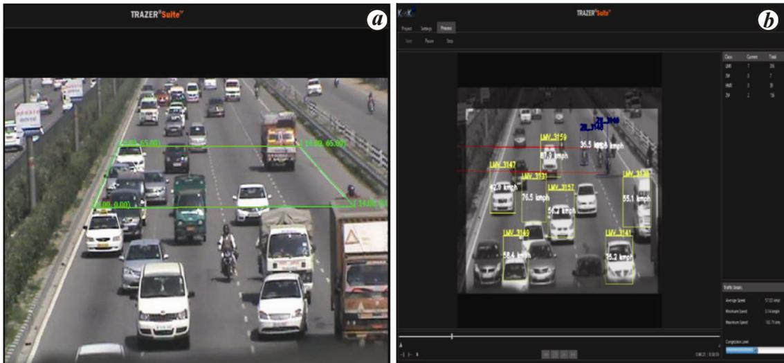
Figure 5. a, Trap length marked on detection window. b, Vehicle detection window of TRAZER.
