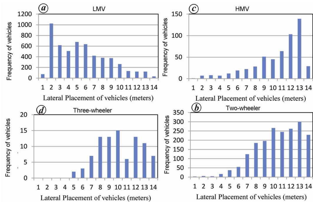
Figure 6. Frequency of vehicles across road width based on their lateral position for (a) light motor vehicle, (b) two-wheeler, (c) heavy motor vehicle and (d) three-wheeler.
