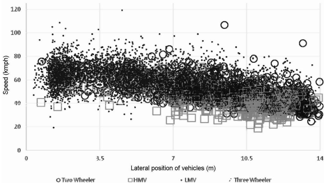
**Figure 11.** Variation in individual vehicle speed with lateral placement for all vehicle categories.
