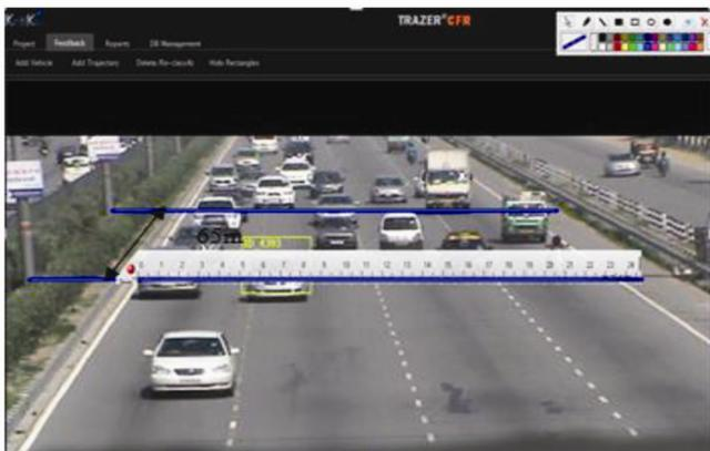
**Figure 4.** Entry and exit lines marked with screen marker and WINDOW RULER used to measure distance across width.
