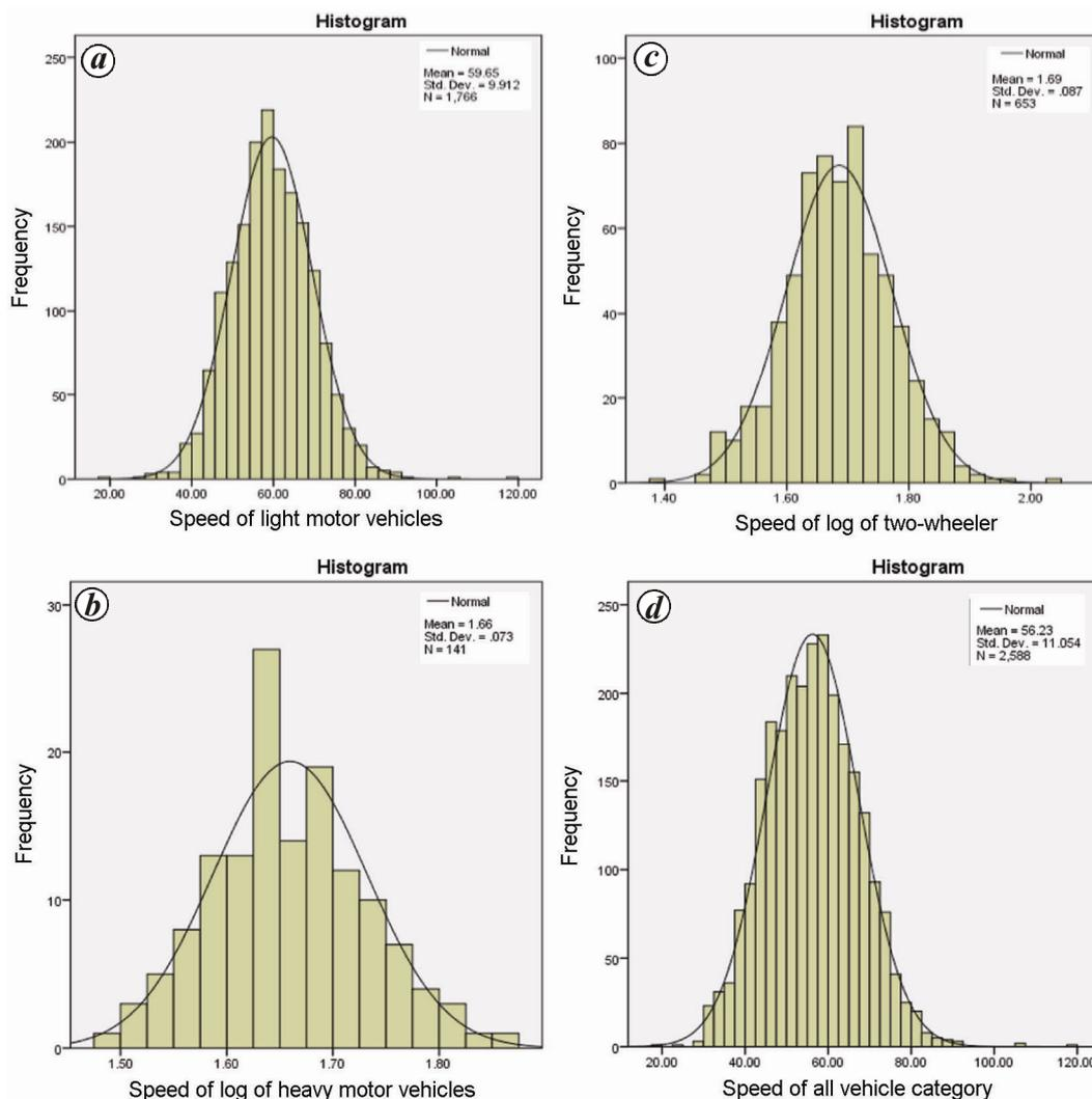
Figure 10. Normal distribution speed fitted for: (a) LMV, (b) HMV, (c) two-wheeler speed and (d) all vehicle categories.
