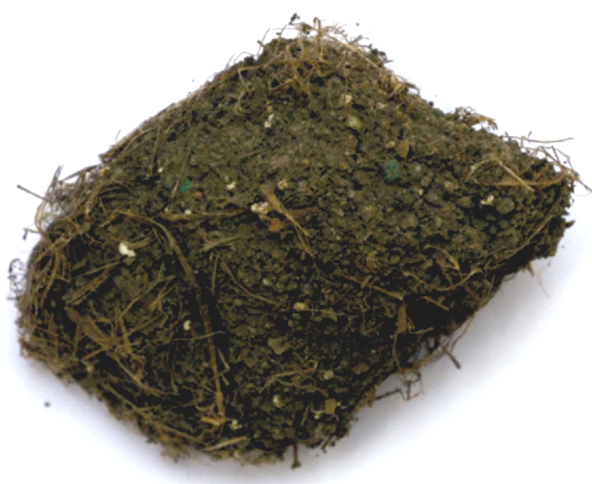
Figure 3. Small piece of clay plaster showing Cannabis fibres.
