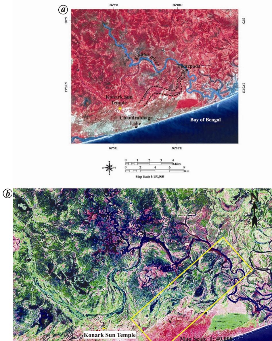
**Figure 2.** *a*, False colour composite image of Konark region depicting the palaeo-channel trace (marked with dashed line) near the Sun Temple. *b*, ETM + Pan mosaic image showing the trace of the palaeo-channel. The yellow rectangular area shows the limits of the present study.
