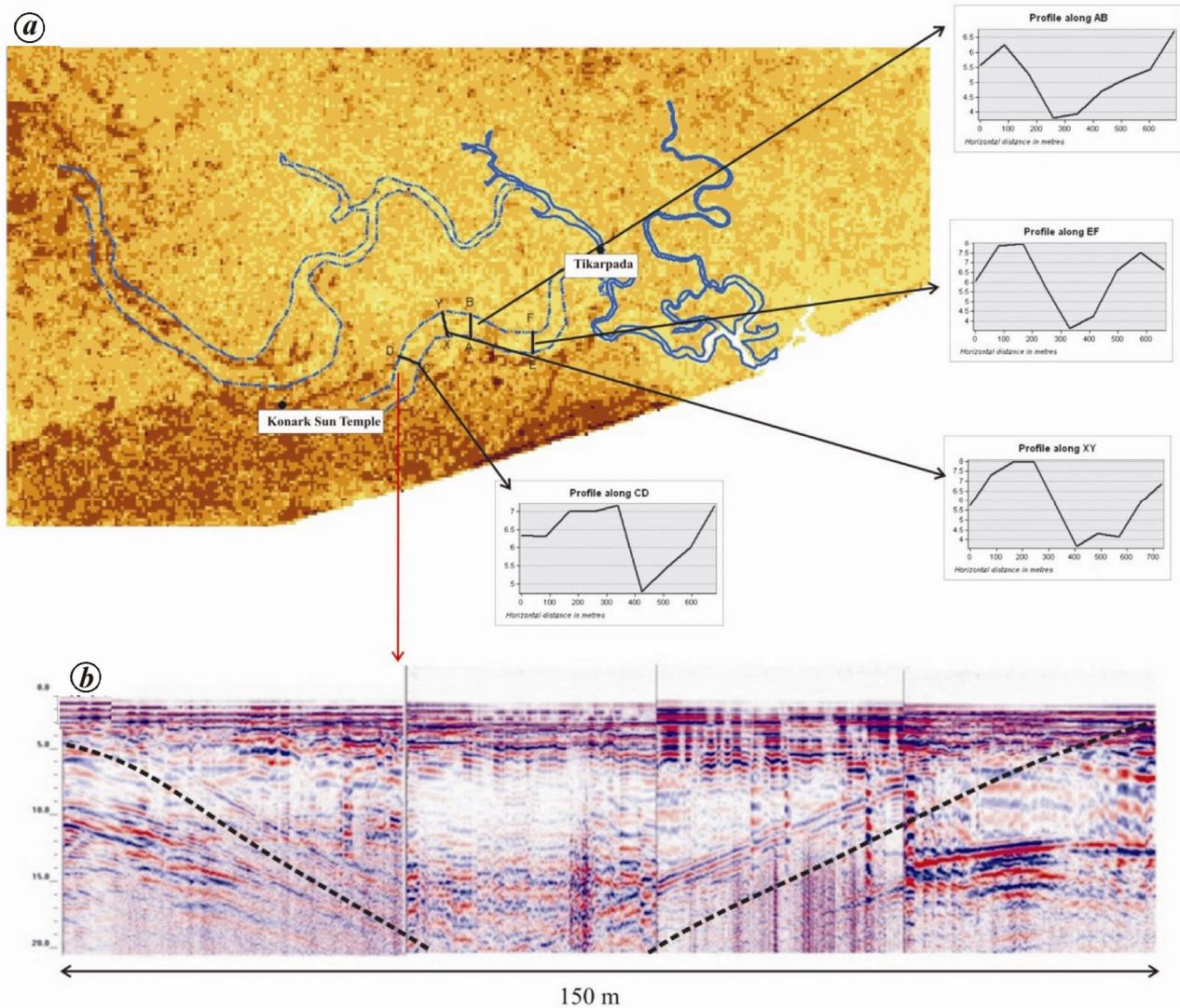
**Figure 3.** *a*, Spatial profile along the selected line traverses across the suspected palaeo-channel, showing its V-shaped topographic outline. *b*, Subsurface image of the river channel inferred from GPR survey along the traverse shown in (*a*).
