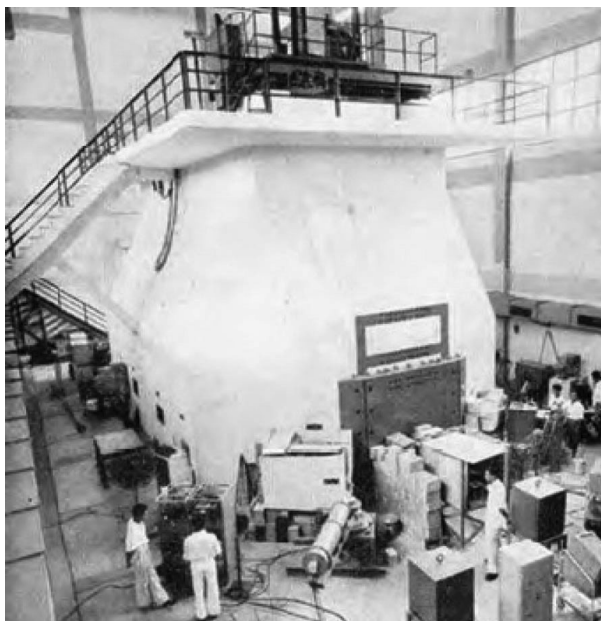
Figure 1. Apsara reactor: neutron diffractometer in the forefront.
