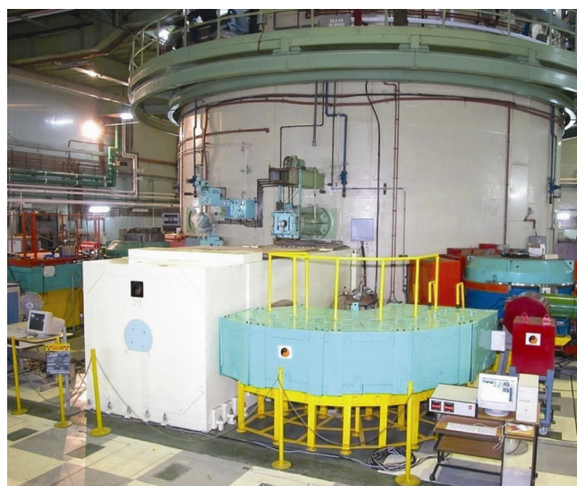
Figure 25. Diffractometer based on multi-monochromator layout. White monochromator shield and green detector shield are seen in the photograph at Dhruva.
