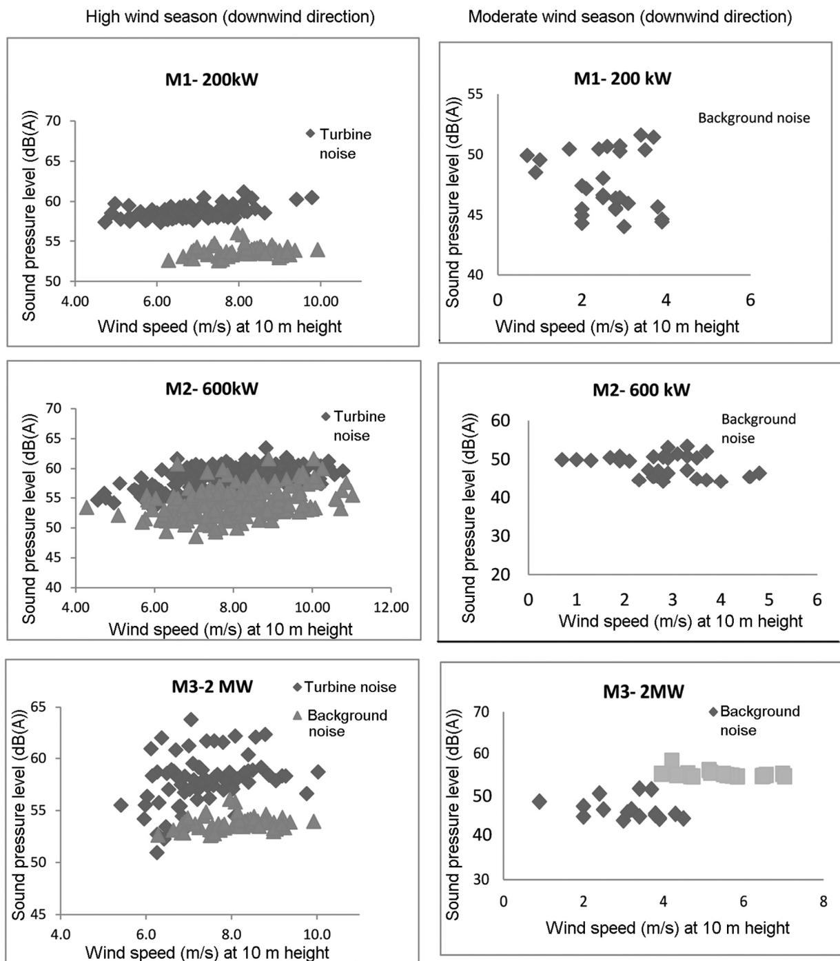
Figure 6. Wind turbine noise studies – high and moderate wind seasons (200 kW, 600 kW and 2 MW).
