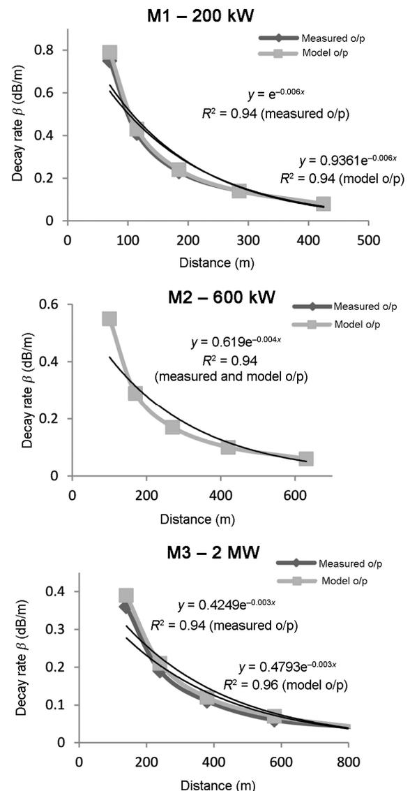
Figure 9. Decay rate for measured and model output for M1 – 200 kW, M2 – 600 kW and M3 – 2 MW.
