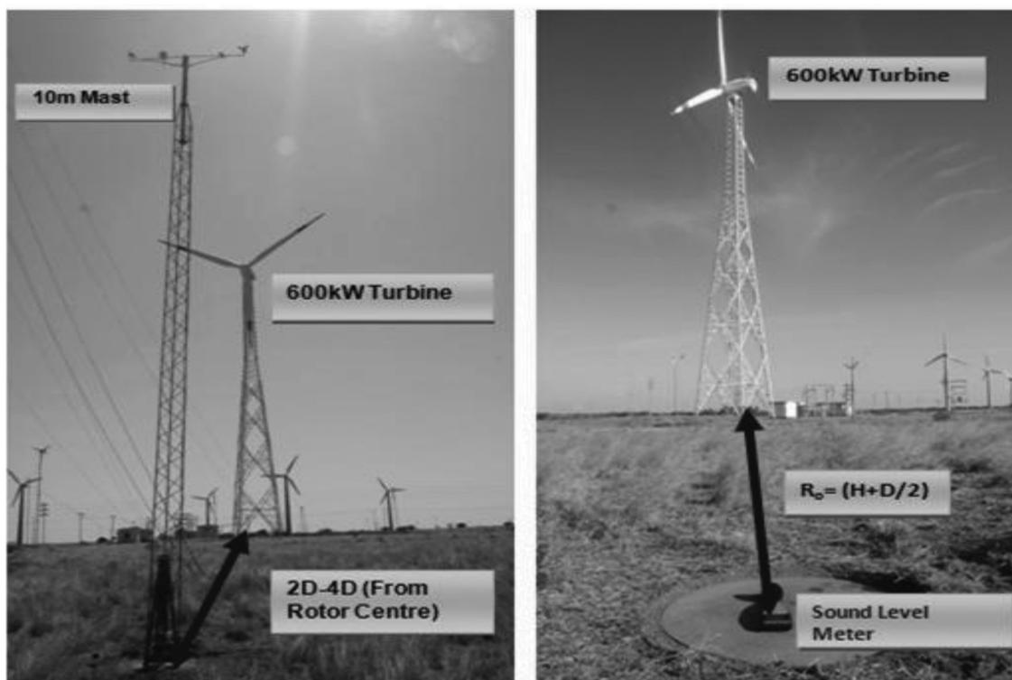
Figure 3. Onsite measurement settings according to IEC 61400-11.
