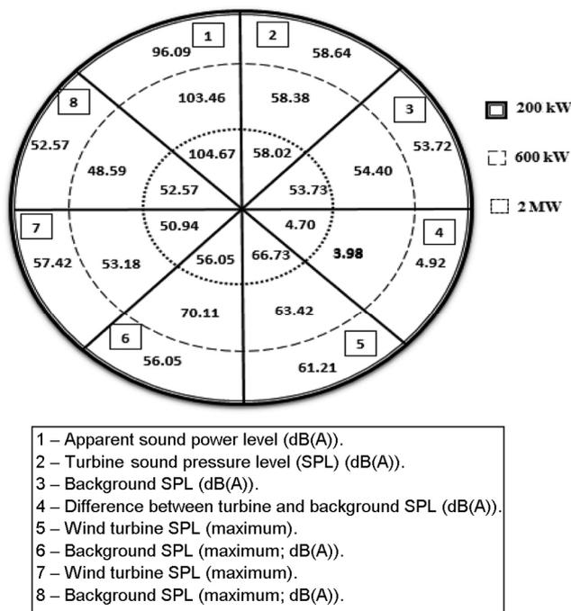
Figure 5. Noise level measurements of three wind turbines.
