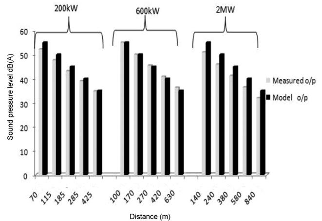
Figure 8. Comparison of wind turbine noise propagation (M1 – 200 kW, M2 – 600 kW and M3 – 2 MW capacity machines).
