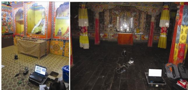
**Figure 10.** Experimental set-up consisting of seismometer and data acquisition system at Enchey and Labrang monasteries.**Table 2.** Frequency measurement of the ambient vibration test
