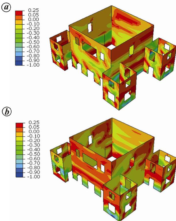
Figure 17. In-plane stress contour plots which identify areas of critical stress: *a*, x-direction; *b*, y-direction.
