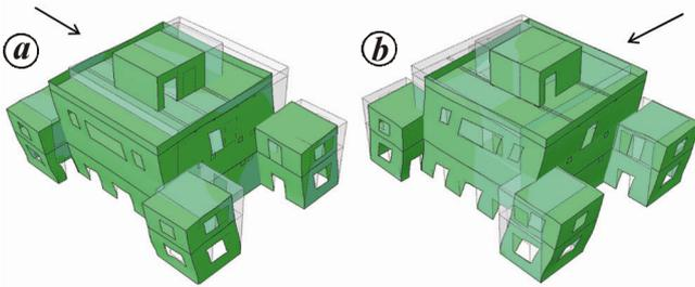
**Figure 14.** Mode shapes for natural frequency: *a*, x-direction; *b*, y-direction.
