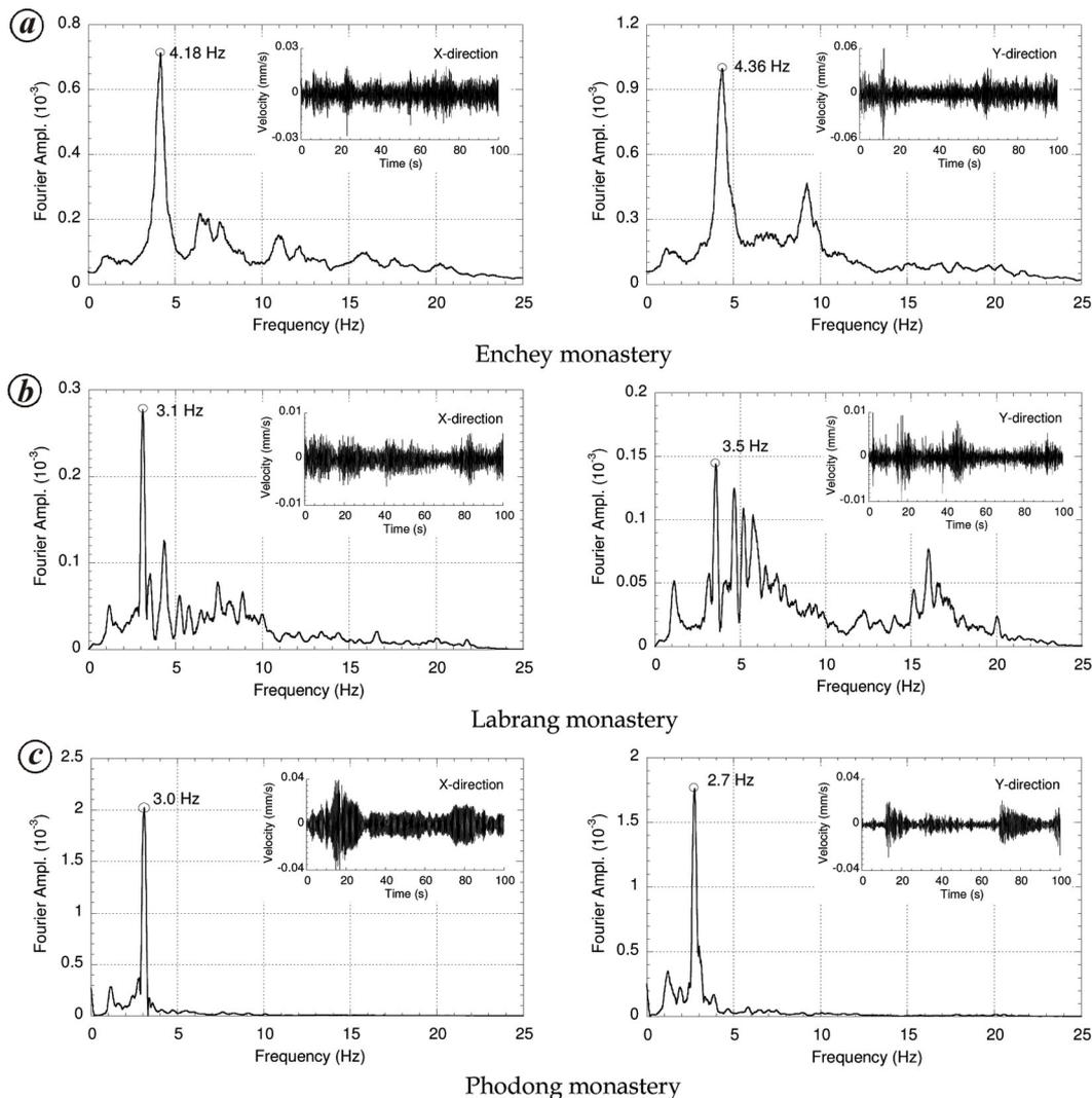
Figure 11 a-c. Recorded time-history and Fourier spectra at three monasteries in the x-direction parallel and y-direction perpendicular to the main entrance.
