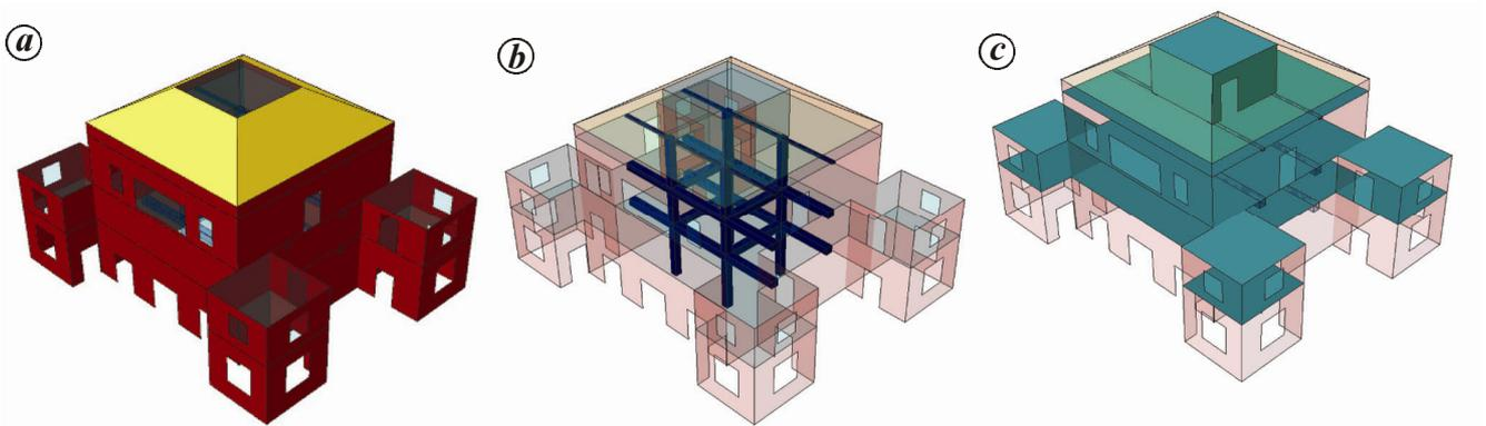
**Figure 13.** View of finite element models: *a*, Exterior masonry walls and pitched roof of GI sheet; *b*, Frame system of the structure comprising wooden beams and column; *c*, Roof and floor diaphragms.
