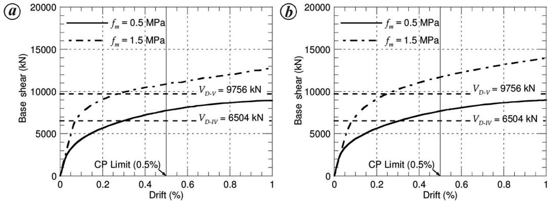
Figure 16. Pushover curve for the Enchey monastery for different masonry properties: *a*, x-direction; *b*, y-direction.
