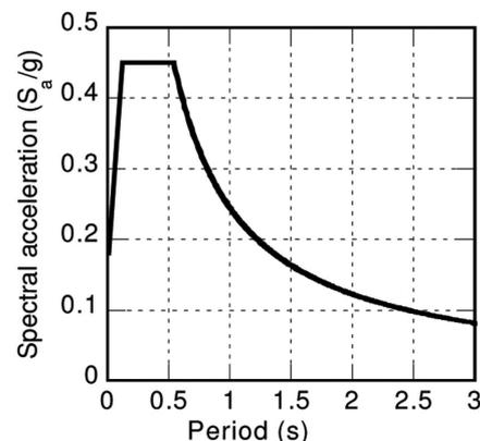
Figure 15. Response spectrum for zone IV soil type II with 5% damping.
