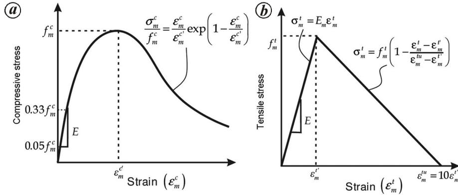
**Figure 12.** Constitutive model of stone masonry with weak mortar: *a*, compressive stress–strain curve; *b*, tensile stress–strain curve.
