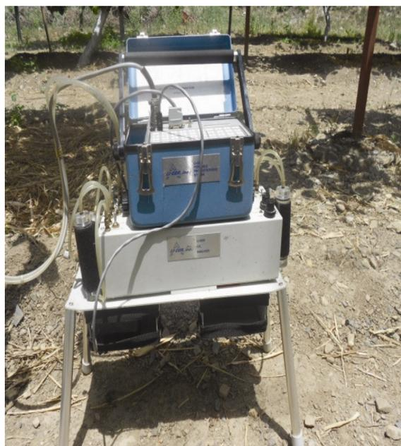
**Figure 3.** LI-COR 6200 portable photosynthesis system.
