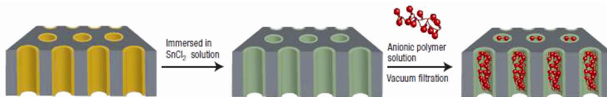
Figure 5. Schematic illustration of functionalization of the nanoporous membranes with polymers.
