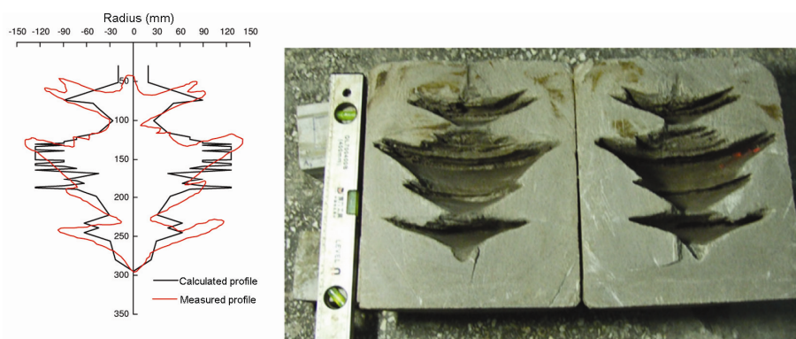
Figure 13. Profile of the cavern constructed in the double-interlayer-containing moulded saliferous aggregates specimen.
