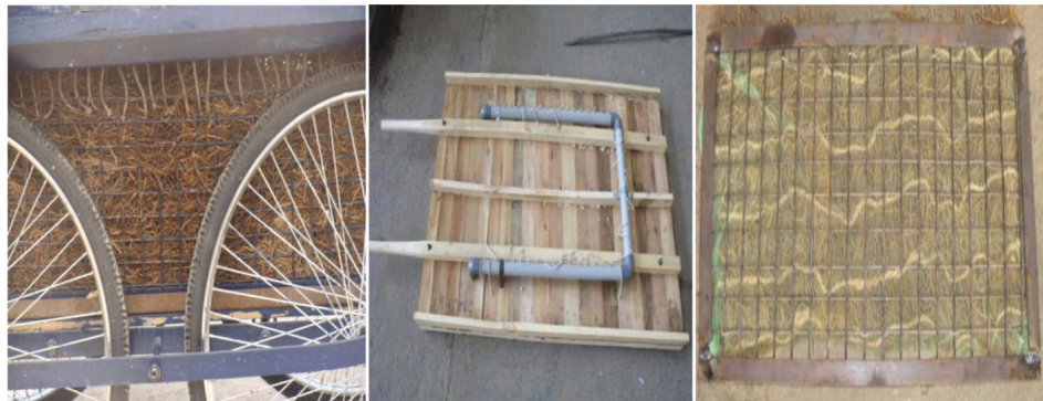
Figure 3. Cotton wick (regulated) water dispersal system.
