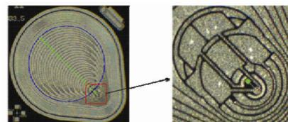
**Figure 2.** Silicon drift detector with integrated FET input stage.
