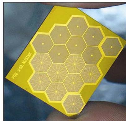
**Figure 1.** Silicon drift detector droplet SD<sup>3</sup>.
