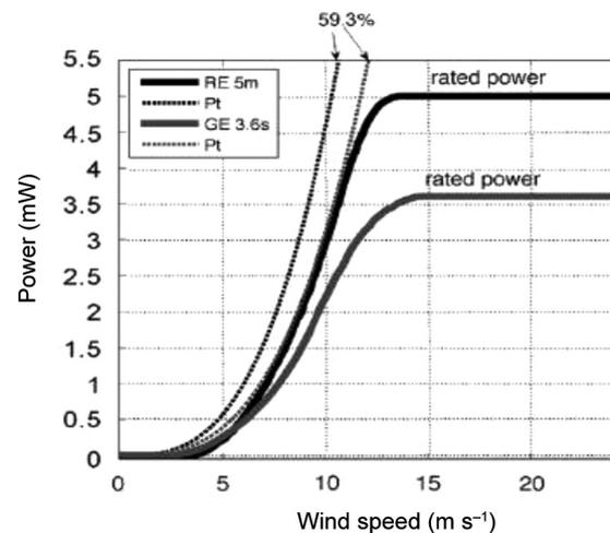
Figure 4. Turbine power curve for GE 3.6s and REpower 5M<sup>17</sup>.
