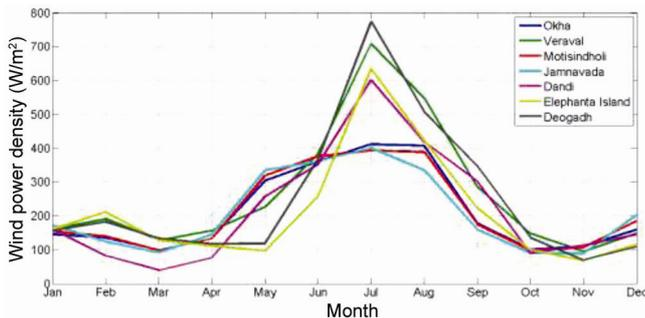
**Figure 3.** Monthly average wind power density at 80 m hub height.
