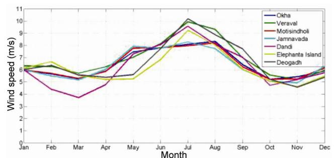
**Figure 2.** Monthly average wind speed at 80 m hub height.
