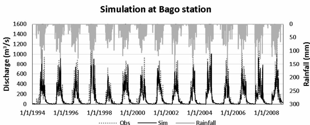
Figure 6. Comparison of observed and simulated daily discharge during calibration at Bago station.
