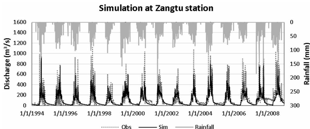
Figure 5. Comparison of the observed and simulated daily discharge during calibration at Zangtu station.
