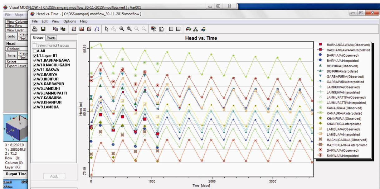
Figure 14. Groundwater behaviour under proposed cropping intensity of 222% for a period of 10 years, if Conjunctive use is implied.
