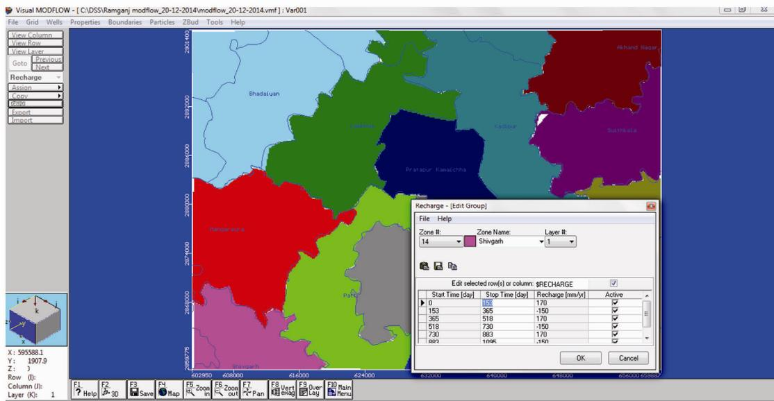
Figure 6. Recharge zones at block level in the groundwater model.
