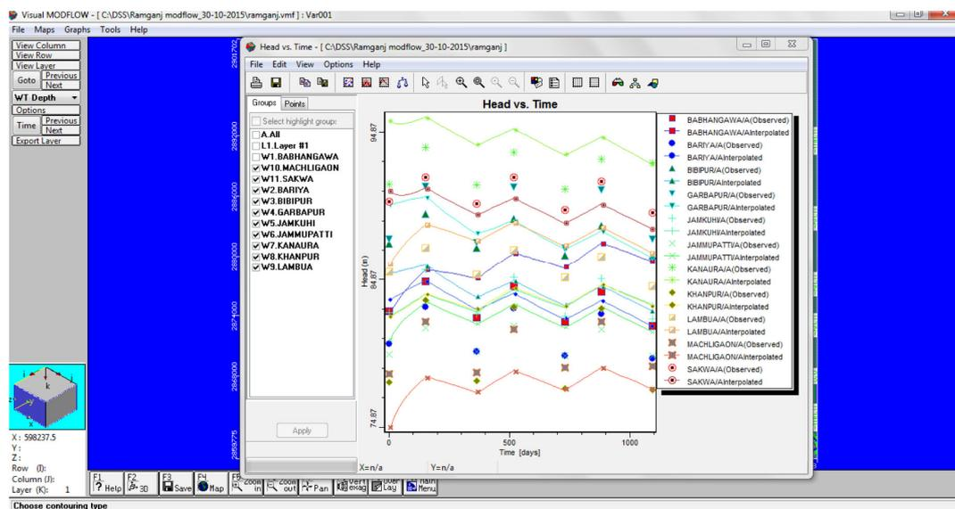
Figure 8. Model calibration run showing the calibrated and actual water levels.
