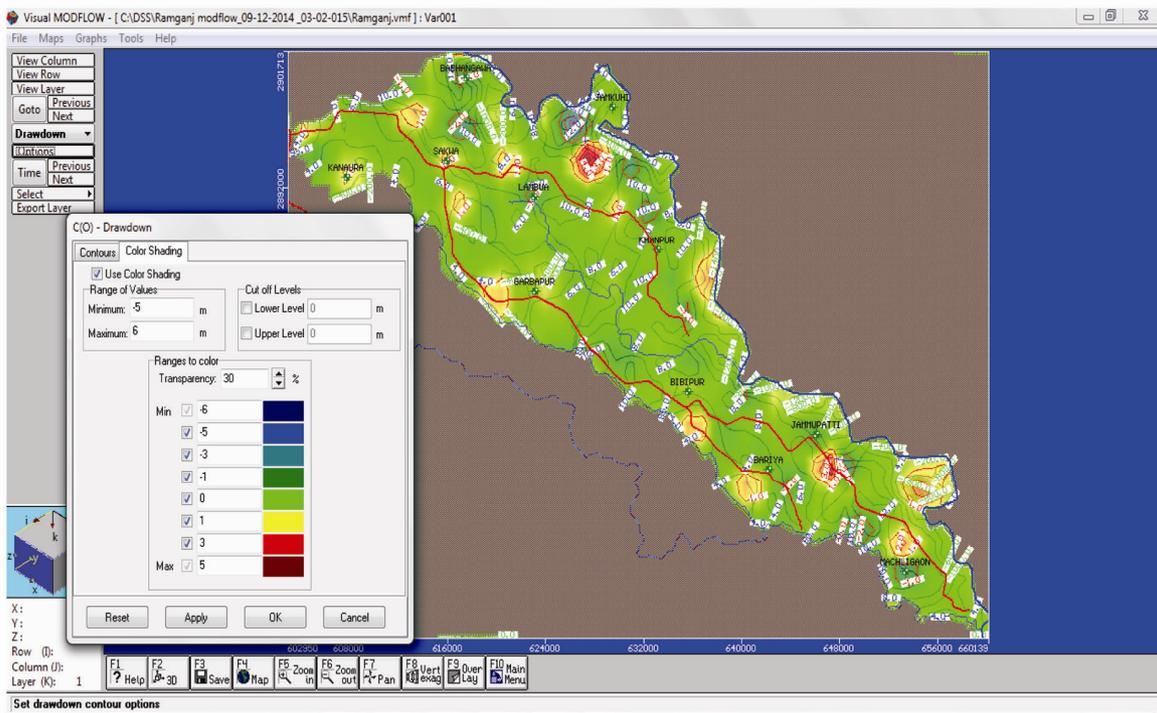
**Figure 13.** Draw-down in groundwater levels under the present cropping intensity of 163.1% during a period of three years, if conjunctive use is implied.
