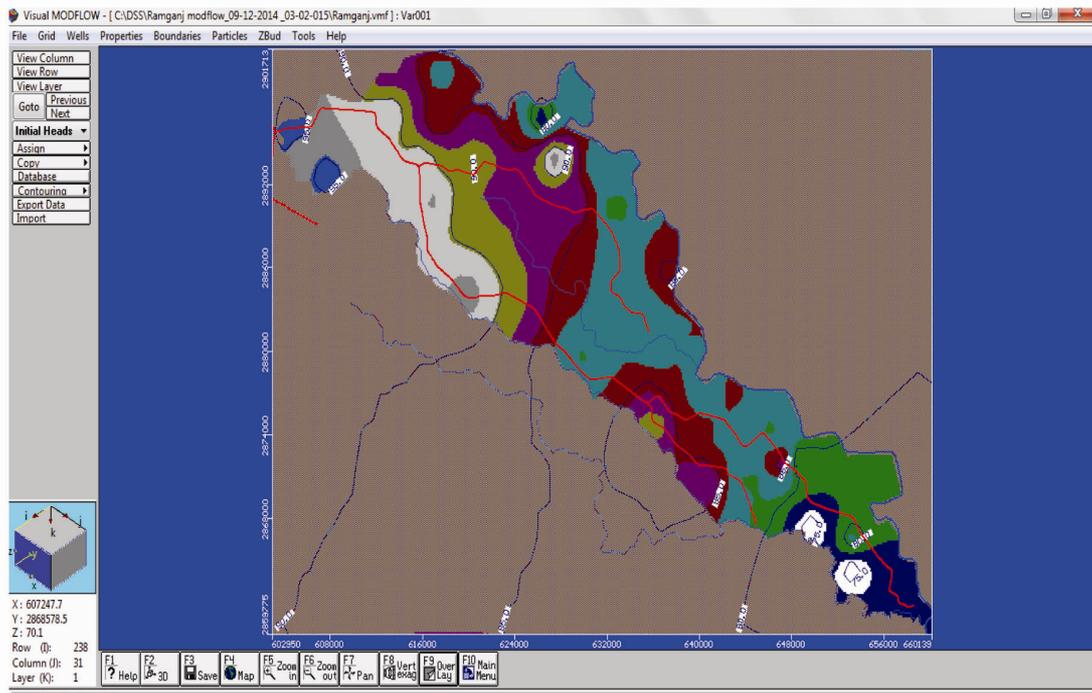
Figure 5. Initial groundwater levels.
