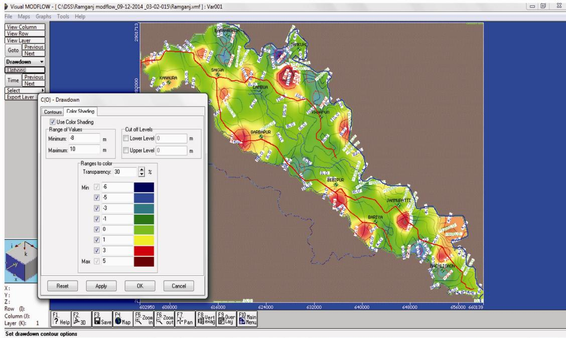
**Figure 12.** Draw-down in groundwater levels during a period of three years under current irrigation practices for the existing cropping intensity of 163.1%.
