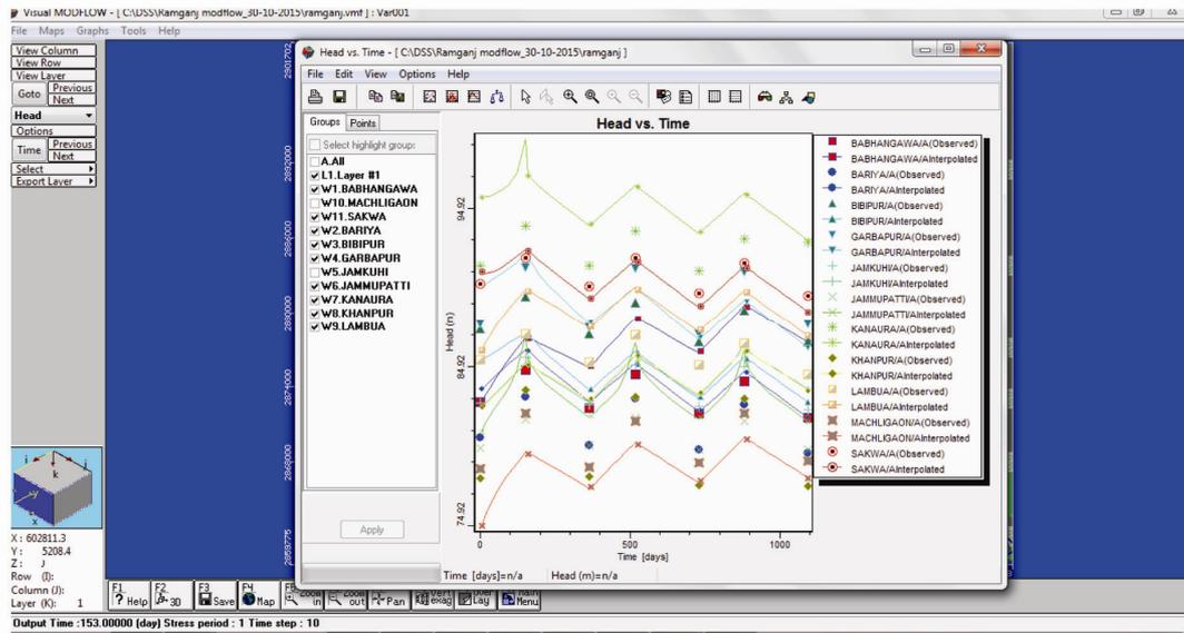
Figure 10. Groundwater levels for proposed cropping intensity of 222%.
