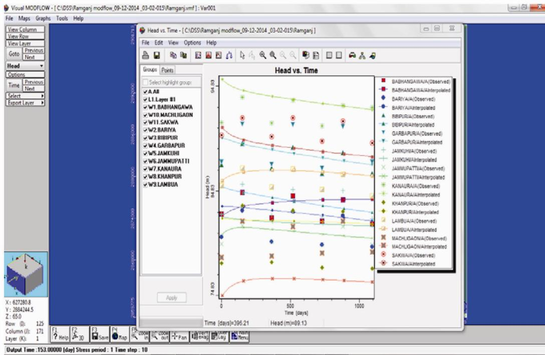
Figure 11. Groundwater levels at the predicted uniform net recharge of -90 mm/yr for the proposed cropping intensity of 280%.
