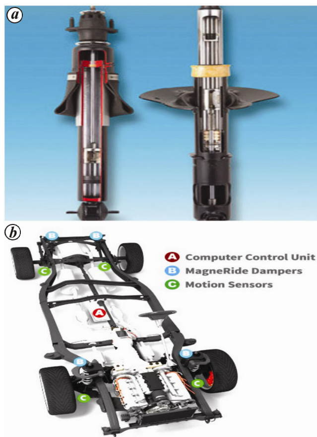
Figure 5. Parts of a MagneRide controlled suspension system 74 . a , Cutaway of a Delphi MagneRide rear shock absorber and a suspension strut. b , The MagneRide system.
