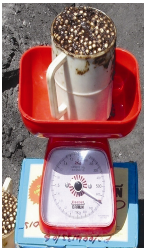
Figure 2. Density measurement of low-density explosive (LDEX) on site.
