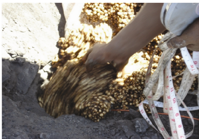
Figure 3. Charging of LDEX into blast holes.
