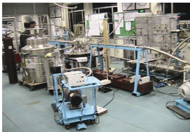
Figure 1. Dilution refrigerator set-up developed in the laboratory.
