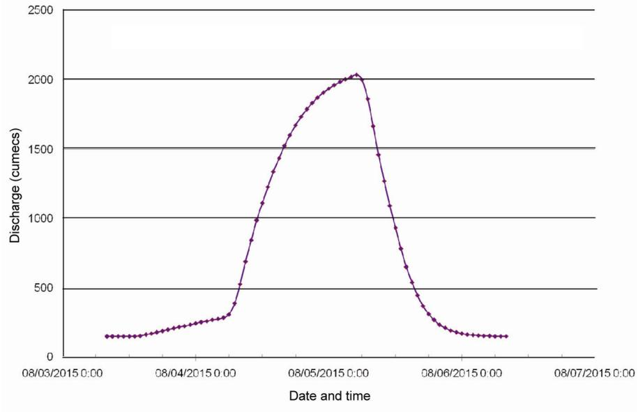
Figure 4. Computed flood hydrograph at rail bridge during the flood event.
