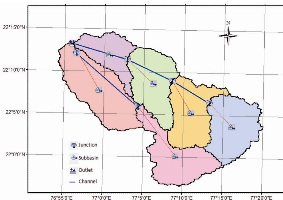
Figure 3. Hydrological model set-up of the study catchment.
