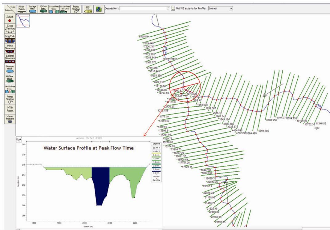
Figure 5. Computed water surface profile and the river geometry.
