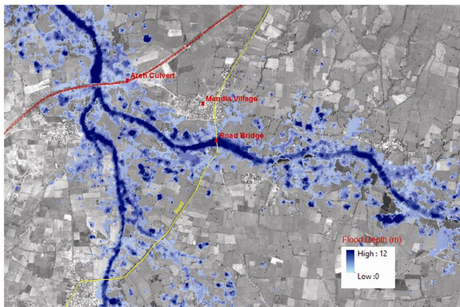
**Figure 6.** Approximate simulated flood inundation during peak discharge in Machak River.
