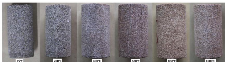
**Figure 1.** Photographs of sandstone specimens after high temperature exposure.
