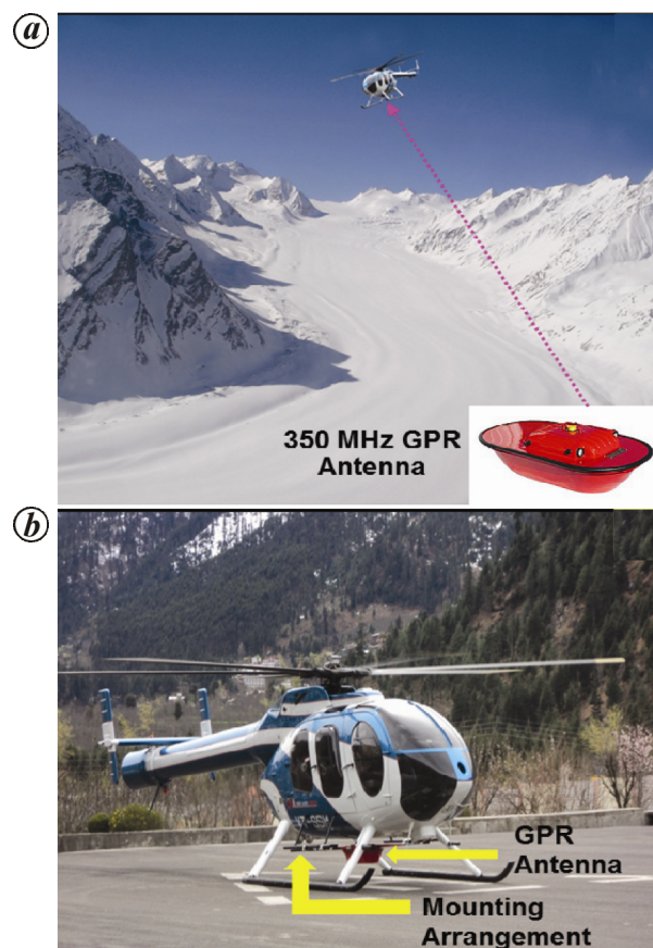
Figure 3. a, GPR centre frequency (350 MHz) antenna mounted beneath a helicopter for airborne data collection over Samudra Tapu glacier in India. b, Air-borne GPR mounting arrangement.
