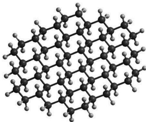
**Figure 1.** Schematic structure of graphane (1.54 Å C-C) layer produced via functionalization of graphene (1.42 Å C-C) with atomic hydrogen (small white balls) in a chair configuration<sup>10</sup>.
