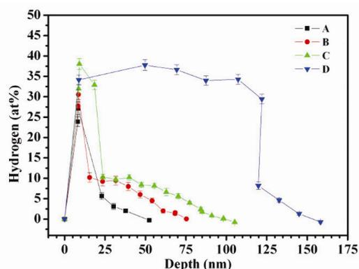
**Figure 4.** Typical depth profiles of hydrogen as measured by ion beam analysis techniques in the 2D-HDLC films (A–D), synthesized under different deposition conditions of  $\text{H}_2 : \text{CH}_4$  ratio.
