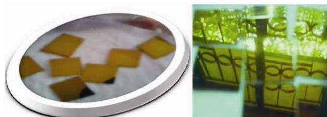
**Figure 2.** Photographs of 2D-hydrogenerated diamond-like carbon (HDLC) films and typical mirror image of surrounding objects due to reflection of light from the films.
