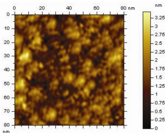
**Figure 6.** Typical STM image of annealed 2D-HDLC film.
