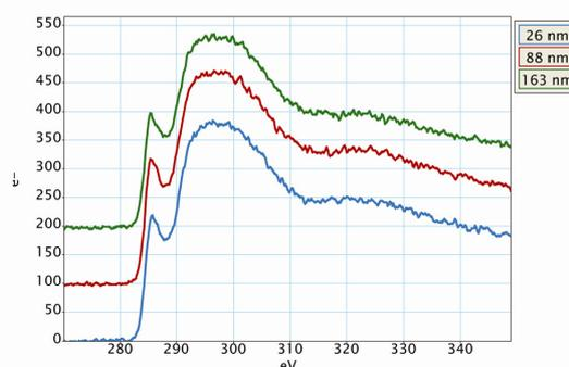
**Figure 3.** Typical electron energy loss spectra of 2D-HDLC film in cross-section geometry at three different depths from the interface of the film-D (vide Figure 4) onto Si substrate.
