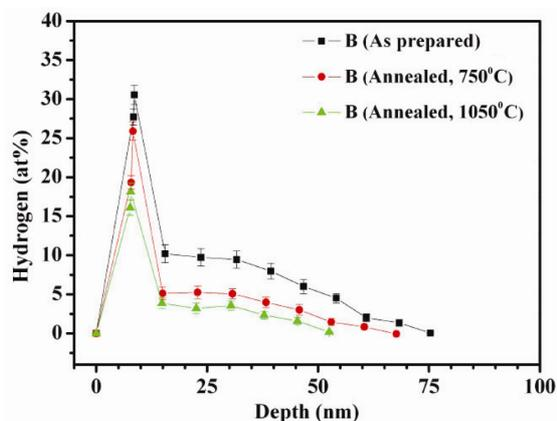
**Figure 5.** Typical depth profiles of hydrogen as measured by IBA techniques in the as-prepared and annealed 2D-HDLC film (film B).
