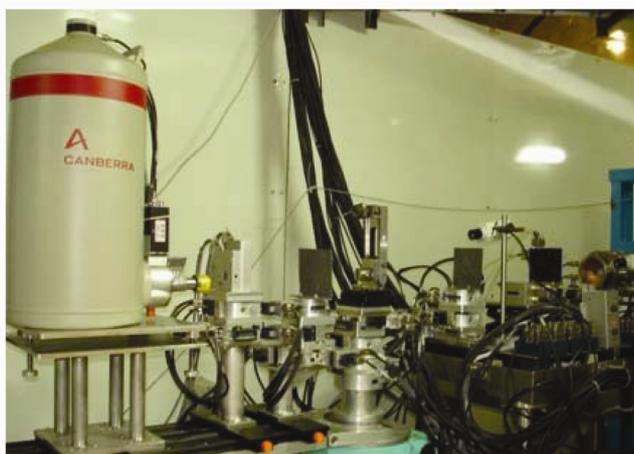
**Figure 8.** Picture showing the ECXRD BL11 beamline at INDUS2 in the energy dispersive mode.
