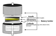
Schematic diagram: Electrochemical cell
