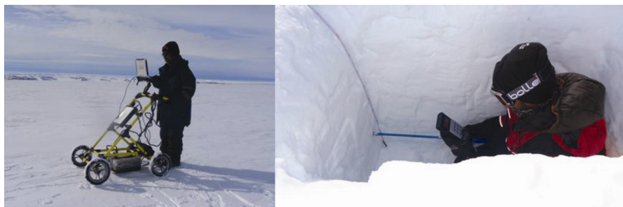
Figure 1. Ground penetrating radar observations over ice sheet and snow fork observations inside the pit.
