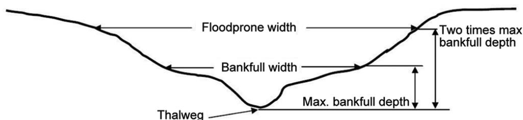
Figure 1. Typical stream channel cross-section for measurement of channel geometry.
