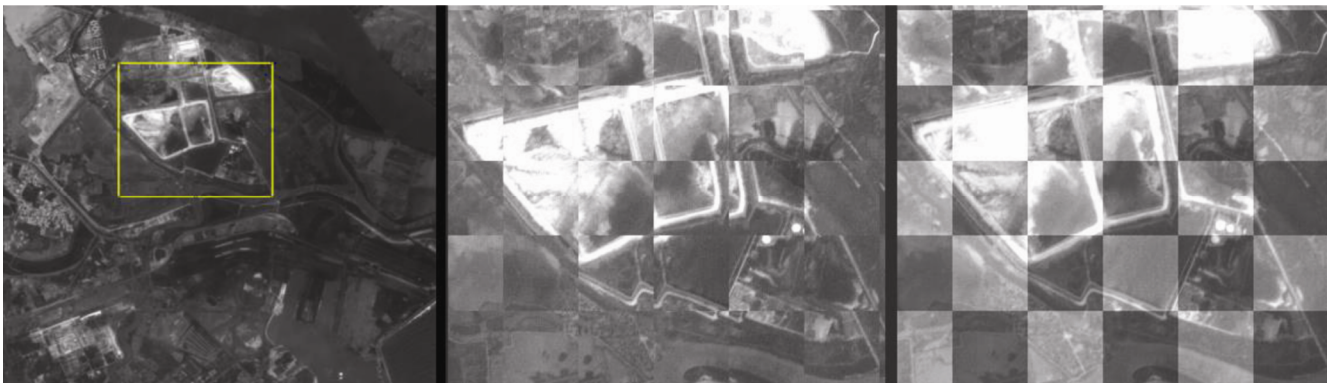
Figure 5. LISS-4 MX B3 sub image (left) and B2 and B3 checker display before (middle) and after (right) registration by only translation.
