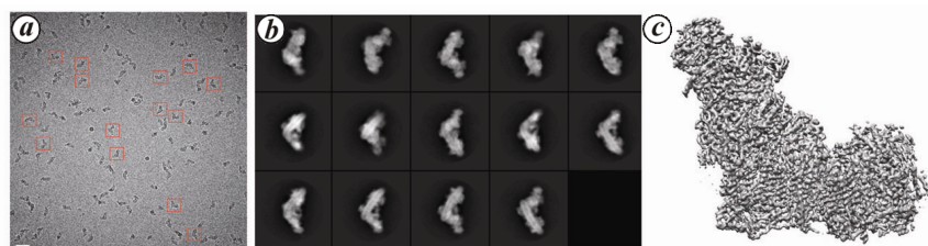
Figure 2. The steps involved in generation of 3D maps of macromolecules by single particle cryoEM is explained with bovine mitochondrial complex I. Protein molecules of interest in solution (complex I in detergent micelles) are rapidly frozen in ethane and imaged with an electron microscope and a direct detector. The micrographs in a show projections of the molecule adopting different orientations on the support film (scale bar is 500 Å). The information content of these images is limited by radiation damage and signal to noise. Many of these projections are then averaged to obtain high resolution information as shown in the 2D class averages ( b ). The box size is 481 Å. The 2D classes of complex I show the TM helices in the membrane domain and densities for accessory subunits. Subsequently, the orientation parameters of individual particles (the three Euler angles and X and Y translations) are determined and a 3D map is reconstructed ( c ). The represented map is the raw data, which is then used to interpret and build model. Figures based on ref. 11.
