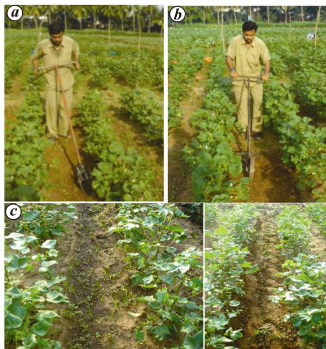
**Figure 4.** Weeding operation in the cotton field. *a*, Twin wheel hoe; *b*, Developed weeder; *c*, Before and after weeding operation.
