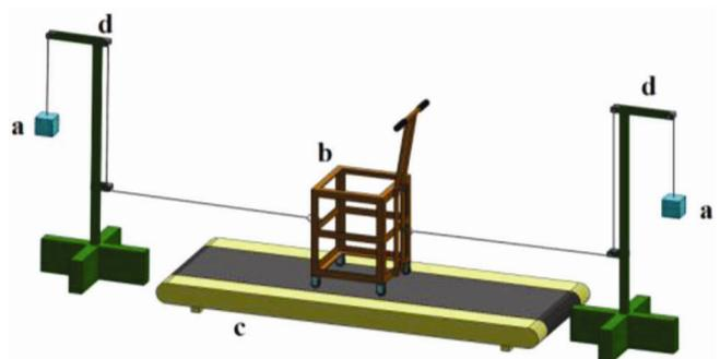
**Figure 1.** Test rig to measure dynamic push–pull strength capabilities. *a*, Varying load; *b*, four wheeled cart; *c*, treadmill; *d*, supporting stands.
