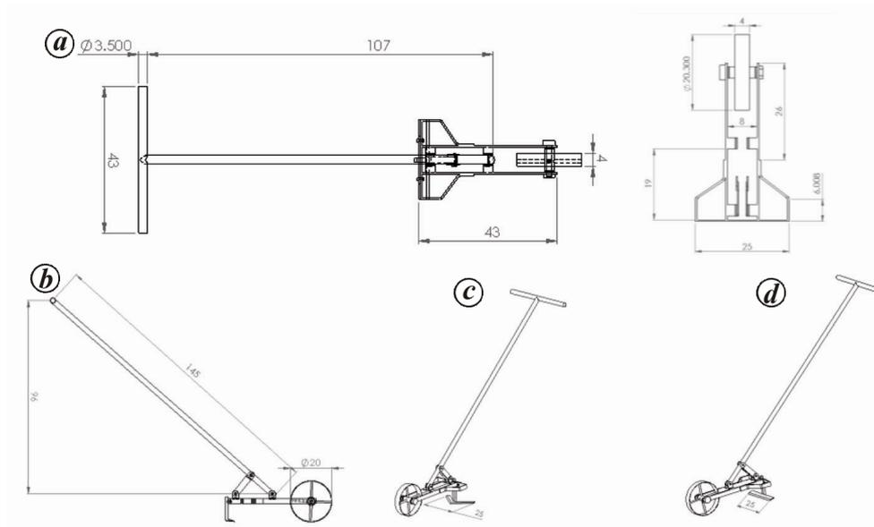
**Figure 2.** Schematic view of the developed weeders. *a*, Elevation drawing of main frame and weeding blade holder assembly; *b*, Plan; *c*, Apex angle 90°; *d*, Apex angle 180° (all dimensions are in cm).
