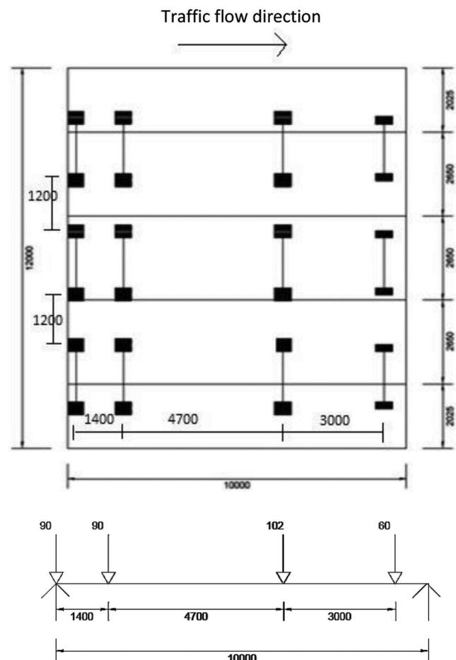
**Figure 4.** Wheel arrangement of actual commercial vehicles on the bridge for maximum shear force.
