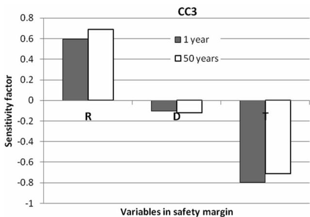
**Figure 6.** Sensitivity factors of variables during 1 year and 50 years for CC3.
