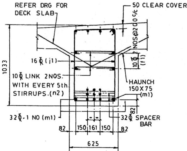
Figure 2. Standard cross-section of T-girder recommended by MORT&H for 10 m.
