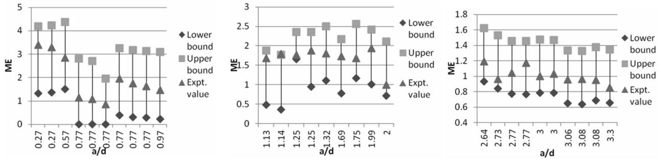
Figure 1. Effectiveness of modelling error in predicting the actual shear capacity for different  $a/d$  ratio.
