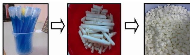
**Figure 1.** Formation of ion imprinted polymer monoliths in tablet form using straws as a mould.
