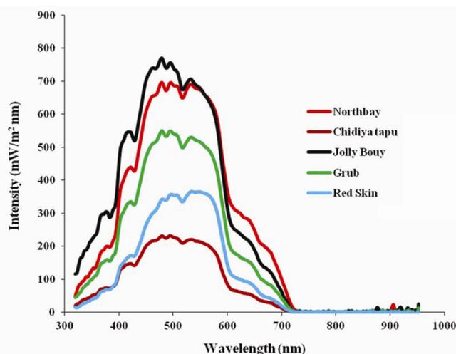
**Figure 5.** Spectral irradiance intensity plot collected at 4 m depth for different Islands.
