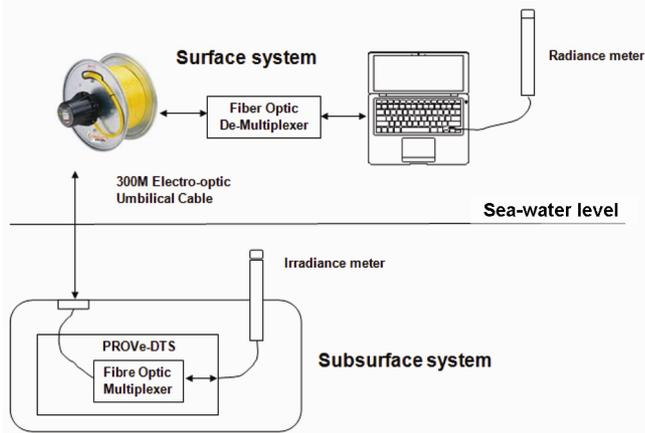
**Figure 2.** RAMSES sensor (radiance and irradiance meter) assembly interface details.
