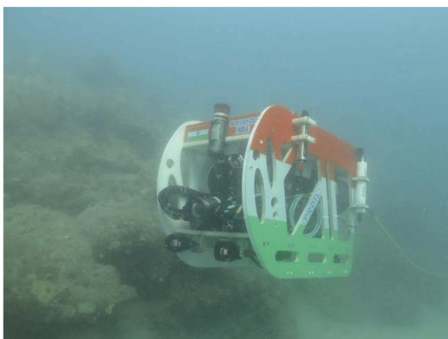
**Figure 1.** Underwater photograph of polar-cum-shallow water remotely operated underwater vehicle (PROVe).
