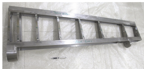
Figure 15. Elevon torsion box made of titanium alloy.
