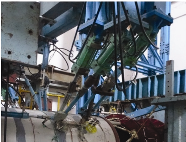
Figure 14. Vertical tail joint load application.
