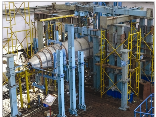
Figure 12. Fuselage static test set-up.
