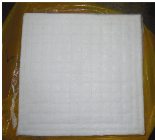
Figure 11. Ceramic-coated FEI after thermo-vac test.
