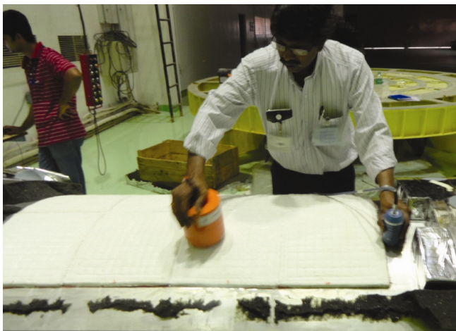
Figure 7. Non-destructive technique inspection for bond integrity after acoustic test.
