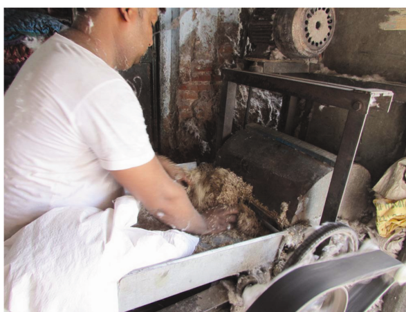
Figure 2. Defluffing of Deenanath grass seed through cotton batting machine.
