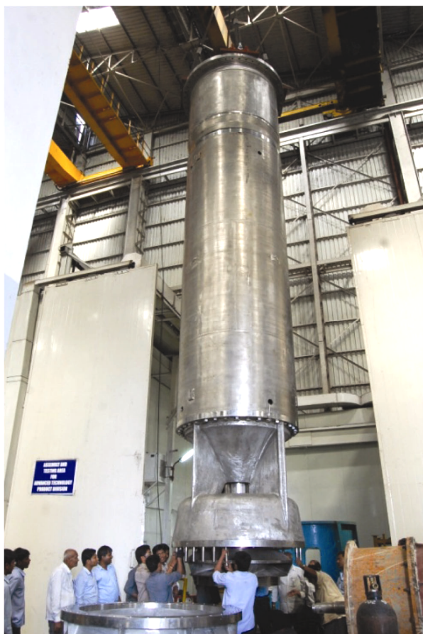
Figure 20. Prototype primary sodium pump being assembled in test bed.
