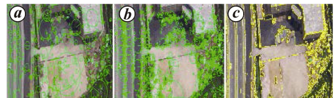
Figure 10. Distribution of the feature frames in scene II. a , SIFT; b , DoG; c , MSER.
