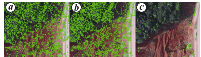
Figure 9. Distribution of the feature frames in scene I. a , SIFT; b , DoG; c , Harris Laplacian.
