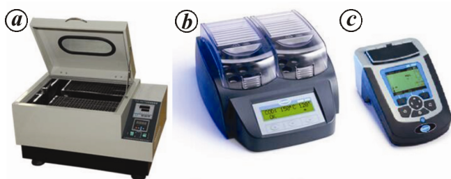
Figure 2. Experimental apparatus. a , The thermostatic shaking gas bath; b , the digestion instrument; c , the visible spectrophotometer.
