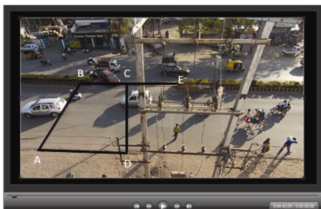
Figure 5. Schematic diagram of influence area for gap acceptance on a 6-lane divided carriageway in Camtasia 8.6.
