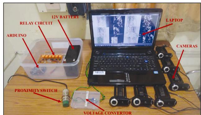
Figure 3. Components of image analysis and controller circuit.
