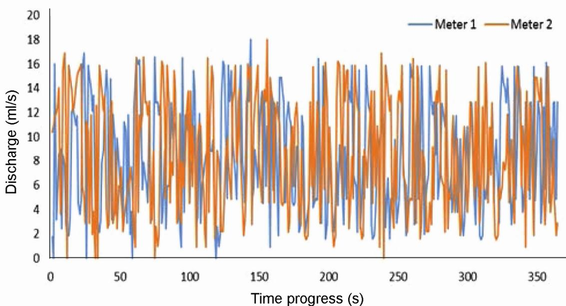
**Figure 13.** Flow variation recorded by the Hall Effect flow meter per variation in weed density.
