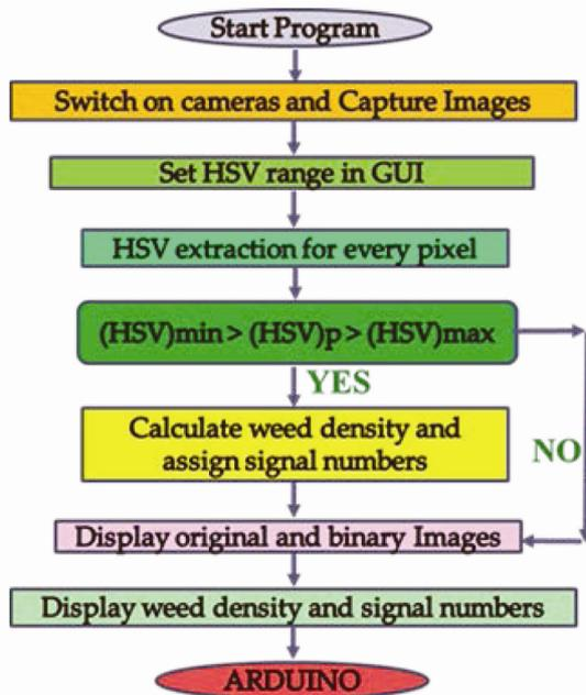
Figure 2. Image analyser process.
