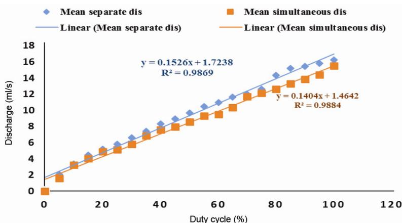
**Figure 11.** Discharge regression for separate and simultaneous solenoid valve calibration.
