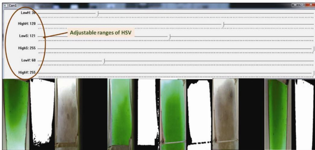
Figure 7. GUI for original and threshold image analysis in laboratory condition with HSV adjustments.
