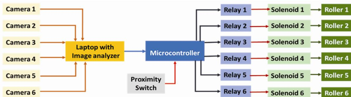
Figure 4. Process flow of the contact-type herbicide application system.
