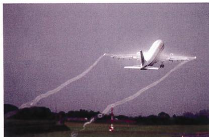
Photograph of the two vortices emerging from the wingtips of an Airbus, made visible by light scattering off water droplets in the vortex cores. Photo © Danel Umaña.
