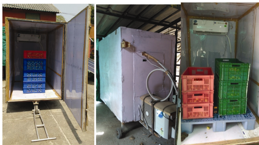
Figure 1. Solar-powered movable cold storage structure connected with 0.8 tonne AC to store tomato.
